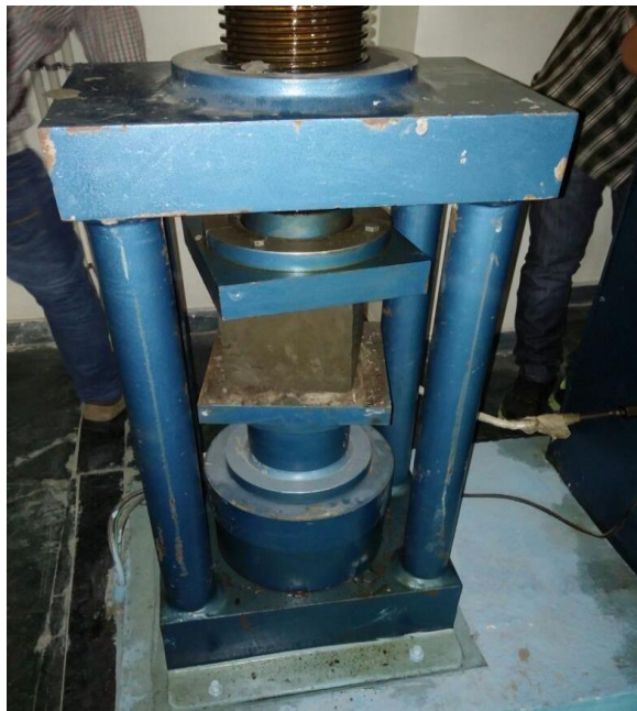
Fig.2. Testing of compressive strength of concrete cubes.
