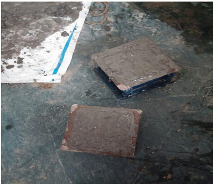
Fig.1 : Concrete with crushed coconut shell as coarse aggregate filled in moulds.
