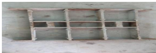
Formwork for moulding of bricks
