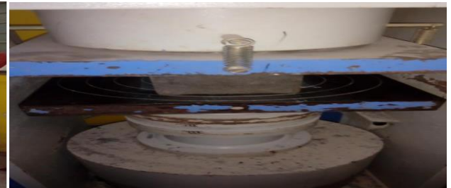
Compression strength test for brick
