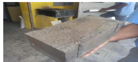
After de-moulding of bricks
