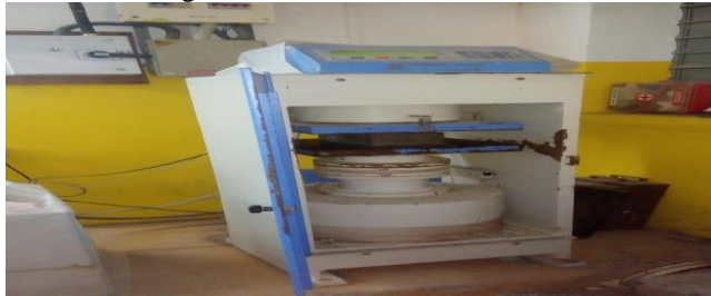
Compression strength test for brick
