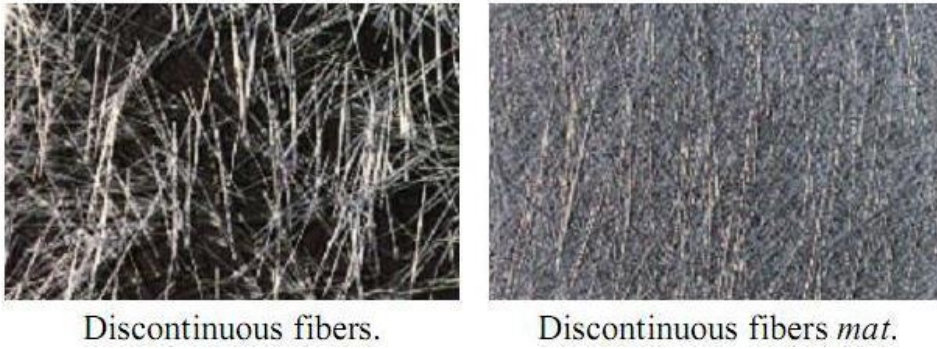
Fig. 2: Discontinuous Glass Fibers
