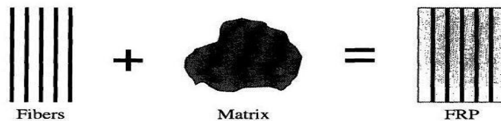
Fig.1: Formation of Fiber Reinforced Polymer Composite
