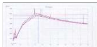
Fig 18: Farinogram of dough prepared from a blend of BsWF and PPPI (protein 25%)
